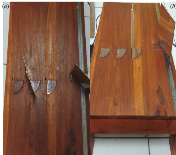
Figure 3. The developed measurement tool to determine the distance between two objects via the law of light reflection, i.e.: (a) top and (b) front views.
